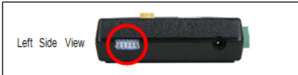
Figure 2. Locating the DIP switch on the Combo Tester X3 and Dual Independent Tester
